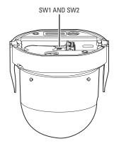
Figure 9. Spectra III Dome Drive DIP Switches
